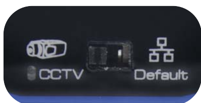
CCTV Mode Switch
