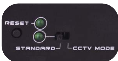
CCTV Mode Switch
