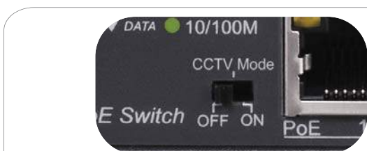
CCTV Mode Switch
