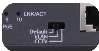
CCTV Mode Switch
