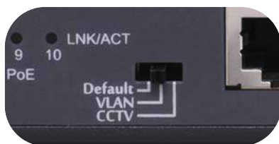
CCTV Mode Switch
